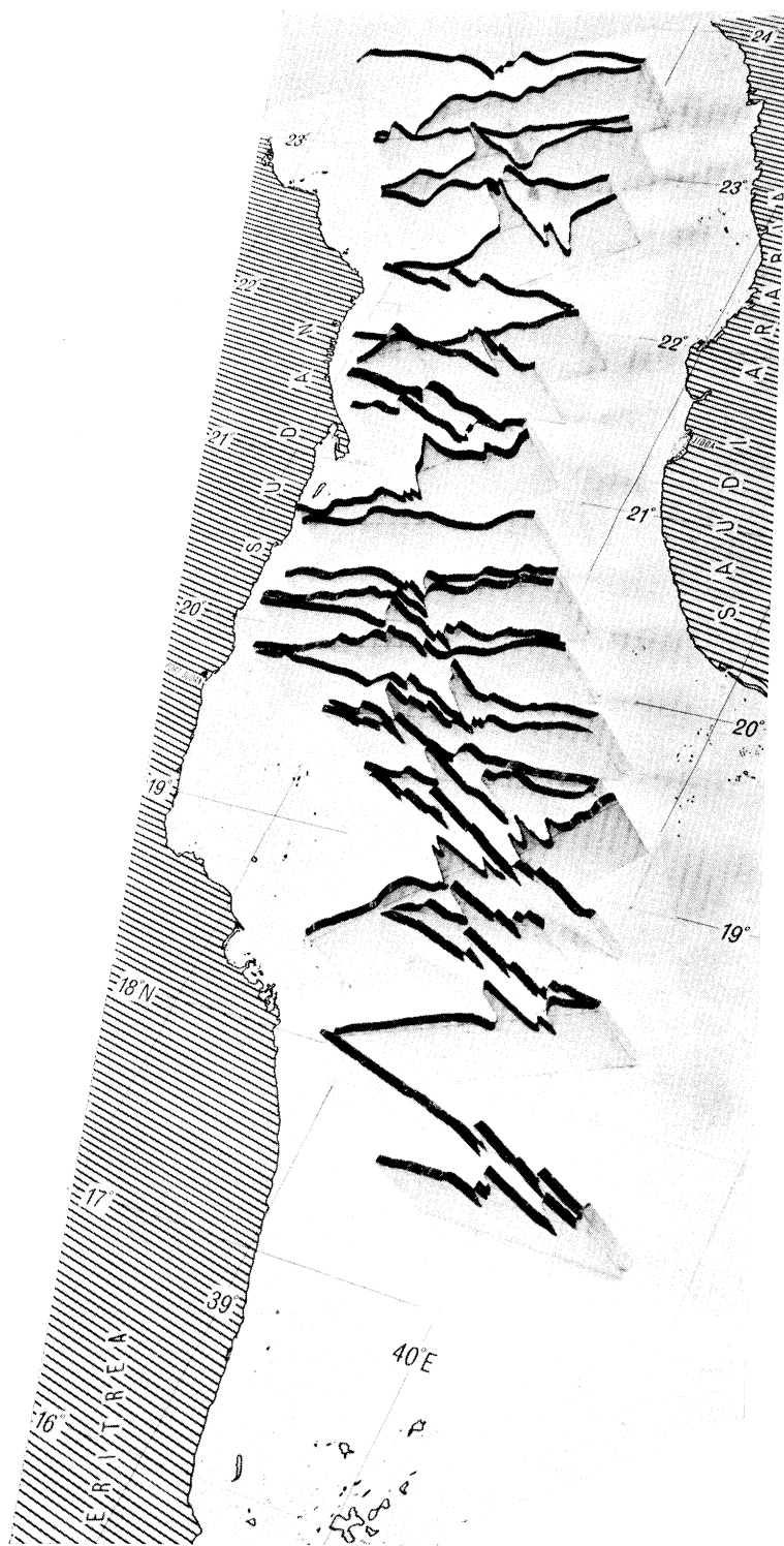
FIGURE 9. Cut-out model of observed magnetic anomaly profiles over the central and southern parts of the Sea.
